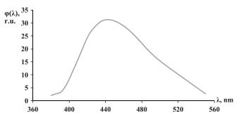
Fig. 3. Averaged photoluminescence spectrum of concentrated mixed fodder
