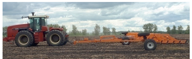
Fig. 4. Machine-tractor unit with an experimental spring harrow during field tests
